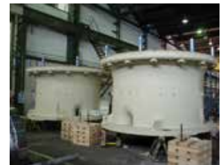
Main frame secondary crusher Bastidor Trituradora Secundaria
