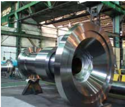
Hydro generator shaft (Ø 2400 mm)
