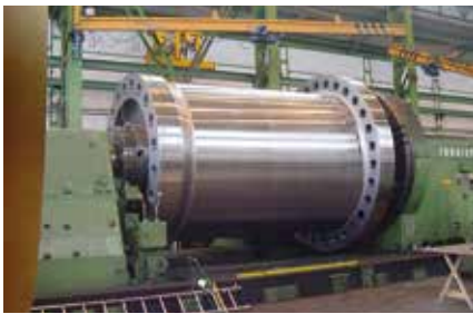
Hydro generator shaft (4000 mm / 110 t)
