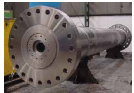
Hydro turbine shaft
