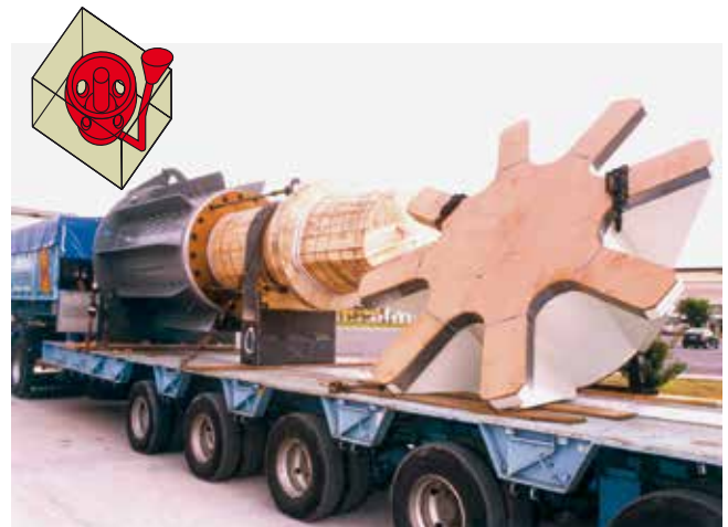
Civil engineering (components for suspension bridges): nodes, connectors, etc Ingeniería estructural (componentes para puentes): nudos, conectores, etc
