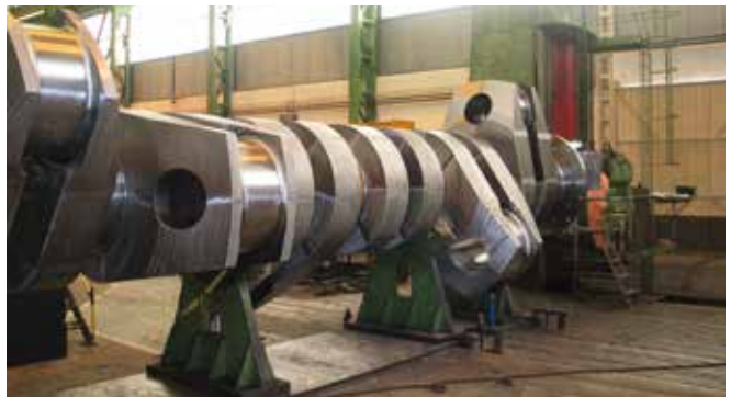
Built-up crankshaft (220 t)
