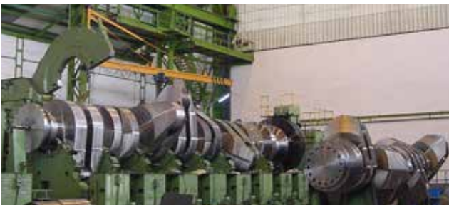
Built-up crankshaft (220 t)
