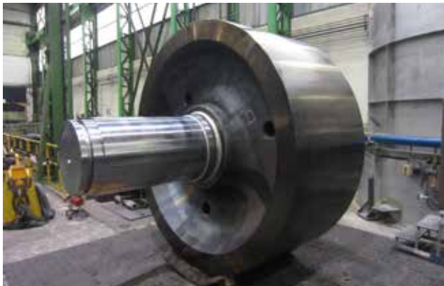
Assembly of roller & roller shaft (shrink-fitting set) Set roldana forjada con eje zunchado
