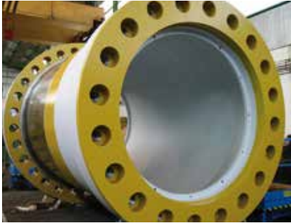
Hydro generator shaft
