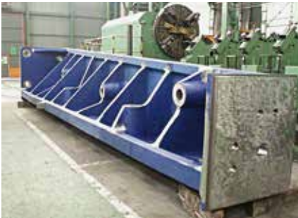
Hammer column section Columna martillo
