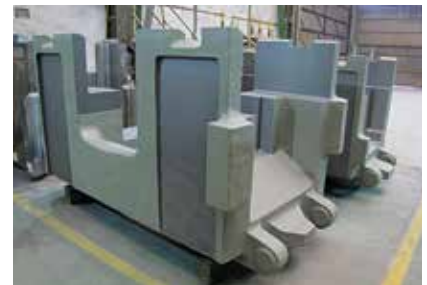
Inferior mill housing Castillete
