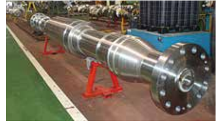
Hydro turbine shaft
