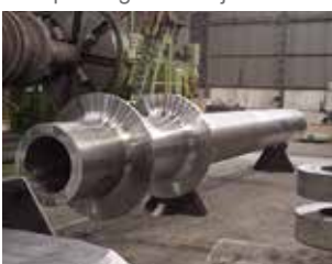
Bucket wheel excavator shaft Eje rotapala
