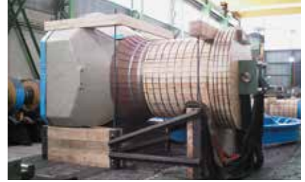
Upper tup (ram) DG-80 (110 t) Maza superior DG-80 (110 t)
